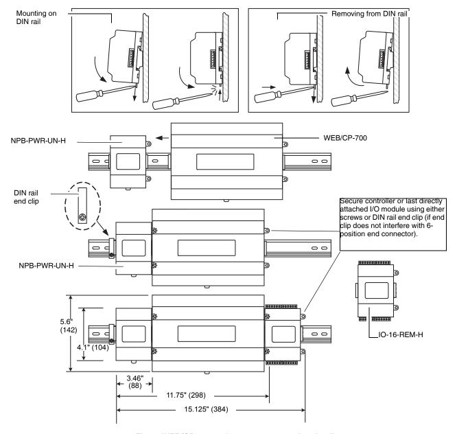
Fig. 3. WEB/CP-700 and accessory mounting details.
